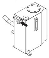
Place a collecting vessel under the tank's drain plug and open the plug.
