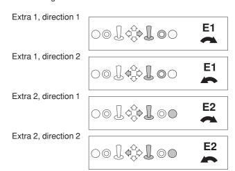
right button on the right joystick is depressed. This can be useful if you simultaneously want to run arm 1 and 2 in parallel.
