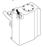
Place a collecting vessel under the tank's drain plug and open the plug.
