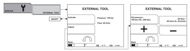
The machine can be used as a power source to operate external hydraulic tools.
