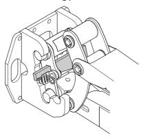
Connect the hydraulic hoses and any hoses for hammer lubrication (when fitting the hammer). Viewed from the rear, the tool's return hose must first be connected to the right side (A port) and then the delivery hose to the left side (B port).
