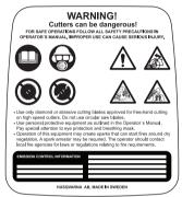
The Emissions Compliance Period referred to on the Emission Compliance label indicates the number of operating hours for which the engine has been shown to meet Federal and California emissions requirements.
