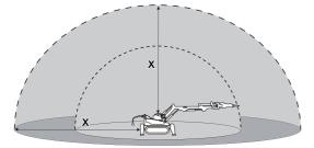
The working area is limited by the machine's reach, however, the risk area varies depending on working method, work object, surface etc. Study possible risks before starting work. If conditions change during the course of the work, the risk area must be redefined.
