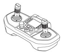
The machine is controlled from the remote control. Transmission of signals is either wireless, using bluetooth, or via a cable.
