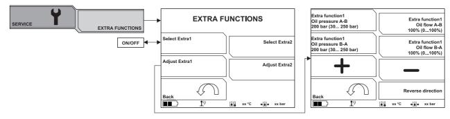
The machine can be equipped with extra valves to make it capable of running more functions, such as a rotor and a tilt.
