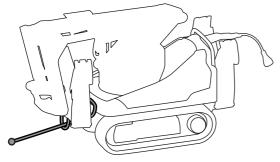
• If possible, retract the outriggers before towing the machine in order to reduce the risk of them getting stuck and being damaged.
