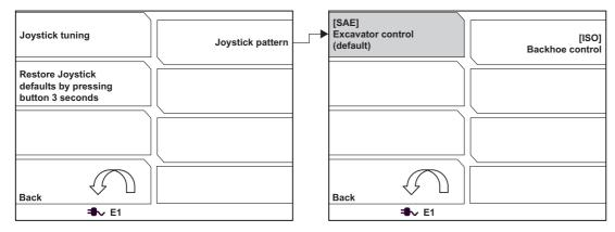
The joystick pattern changes the operation of the remote control. The operational pattern changes as below when the [ISO] Backhoe control is selected.
