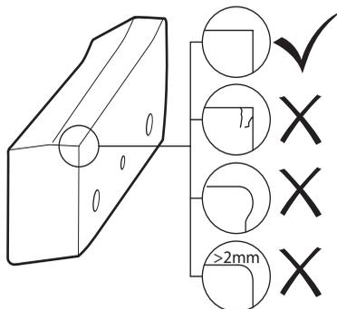
**NOTICE!** Damaged shearers can cause damage to the tool. Never use cutters that are cracked or damaged.
