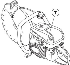
Rec. idle speed: 2700 rpm
