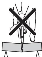
If the blade is pinched or stalled in the kickback zone, the reactive force will push the power cutter up and back towards the user in a rotating motion causing serious or even fatal injury. Be alert for potential movement of the work piece.
