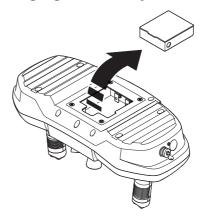
Before using the remote control for the first time the battery has to be charged.
