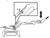
Cylinder 3 is in its outer position and the hammer is working in the downward direction. Never operate the cylinders to their end positions.
