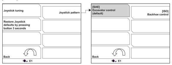
The joystick pattern changes the operation of the remote control. The operational pattern changes as below when the [ISO] Backhoe control is selected.
