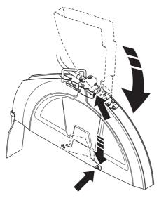
NOTICE! Do not operate this saw without the latch engaged and the bolt installed. Do not use if damaged.
