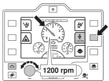
· Set the Engine throttle knob to maximum rpm.
