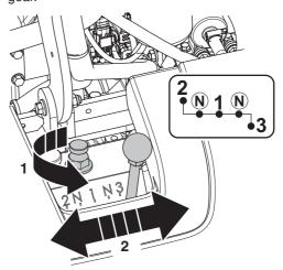
Hand tight knob. Tighten jam nut (30 ft-lbs / 40 Nm).
