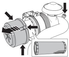
Clean the filter by blowing the element from inside out.
