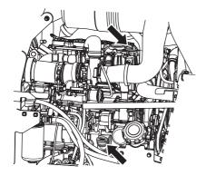
Check the engine's oil level, see instructions under heading "Daily maintenance".
