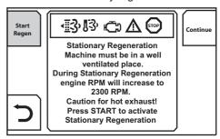
Let the machine cycle rpm and regenerate the DPF (25-30min)
