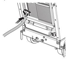
· Close the valve and refill the radiator coolant.
