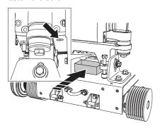
Refill the system by removing the left screw and pour oil into the tube. Look in the window and fill until the correct level is reached.
