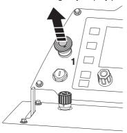
Reset the safe mode by turning Engine start switch to the STOP position and back to ignition on position.
