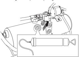
Replace the hydraulic system filter. Fill the new filter with oil and lubricate the seal with a few drops of oil prior to refitting it.
