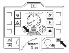
Set the desired cutting depth by rotating the Depth knob.
