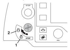
NOTICE! If the engine does not start, turn Engine start switch to STOP position and check the display for any messages. If none, repeat above steps. Else, take measures according to message in the display prior to new starting attempt.
