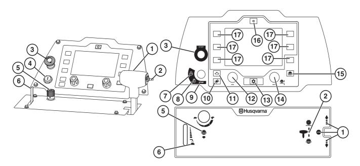
The control panel is the operator's link to the machine. From here the operator can control anything from engine rpm, cutting depth of the blade and read the current status of the engine and the machine.
