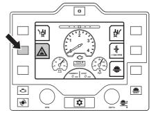
Engage the Blade clutch (if equipped) to engage the blade drive. Only at 1200rpm or less.
