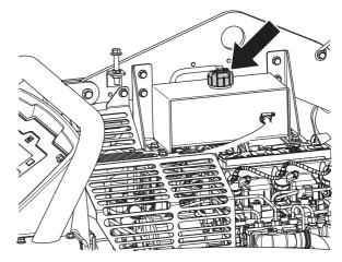
The coolant level should reach the start of the tube inside.
