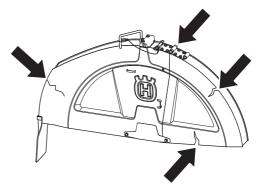
Never use broken or damage blade guard.
