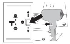
NOTICE! Check to be certain, the transmission bypass valve is closed in the down position.
