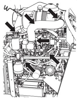
Look for leakage on fuel, hydraulics and cooling system.
