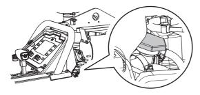
Fill up until the coolant level is between the two marks on the radiator coolant overflow bottle when engine is cool.
