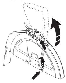
Open the Water valve on the control panel. Make sure it is straight jets of water out of the holes from the water pipes on both sides of the blade and no leakage. Replace water pipe if damaged.
