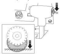
CAUTION! When lowering the blade into a partial cut, align the blade exactly with the cut to prevent damage to the blade.
