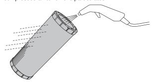
Replace any damaged filters or gaskets and check air hose and clamps for damages or looseness. Tighten or replace as required.
