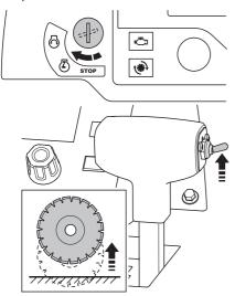
Put Speed control lever into the STOP position.
