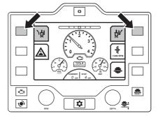
By pressing the E-track zero button on the control panel the rear axle will return to predefined center angle.
