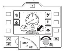
When the blade is lowered the current cutting depth will be showing the difference between the reference point and the diamond blade.  The saw will not lower to any depth greater than the stop position set in the display. If a deeper cut is required, turn the Blade depth knob to a new depth position. You can also disengage the Blade depth stop by pushing the Blade depth stop button to override the depth stop feature.
