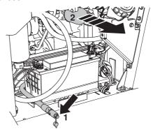
Refill the system at either of 2 locations on the engine.
