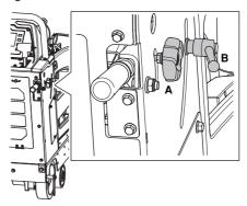
Lower the front guide and align the front guide, rear guide and the diamond blade with the line on the surface. The front guide is telescopic, adjust the length with the screws on the inside of the front guide.
