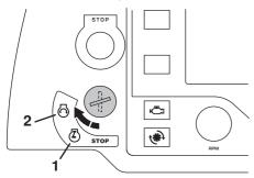
Let the engine warm up for several minutes with Engine throttle at idle speed (minimum).
