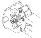
Connect the hydraulic hoses and any hoses for hammer lubrication (when fitting the hammer). Viewed from the rear, the tool's return hose must first be connected to the right side (A port) and then the delivery hose to the left side (B port).
