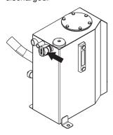
Place a collecting vessel under the tank's drain plug and open the plug.
