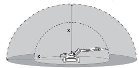
The working area is limited by the machine's reach, however, the risk area varies depending on working method, work object, surface etc. Study possible risks before starting work. If conditions change during the course of the work, the risk area must be redefined.
