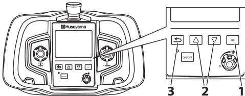
The menu system for the remote control can be accessed by pressing the "OK" button. The menu system comprises the following submenus:
