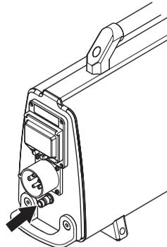
The other water connection should be connected to the power tool, the power tool has various regulating taps for regulating the flow of cooling water to the tool. See the operator's manual for the respective power tools.
