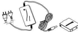
Charging time for a flat battery is approx. 2-3 hours. The diode is orange when charging starts and becomes green when the battery is fully charged. When the battery is fully charged the charger supplies the battery with maintenance current until the battery is removed from the charger.
