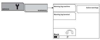
The machine has 2 warning logs and a list of active warnings.
