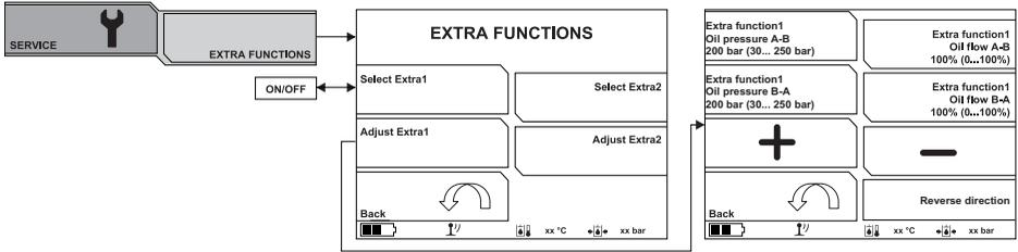
The machine can be equipped with extra valves to make it capable of running more functions, such as a rotor and a tilt. The value for oil pressure and oil flow can be adjusted from port A to B and vice versa. Select which setting you would like to change with the selection keys. Use the arrow keys to change the value.
