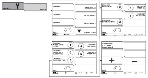
DXR equipped with an Dust Reduction kit enables the water function. The function can be activated together with various tools.
