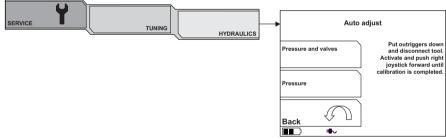
For auto adjustment, the machine should be standing on the outriggers and the tool should be disconnected.
