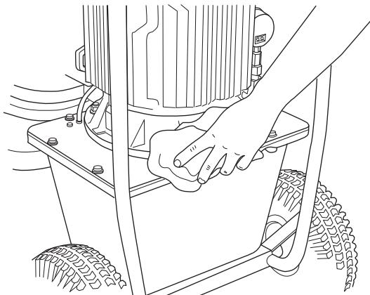
**CAUTION!** Do not use a high pressure washer to clean the power pack. Do not wash the machine with water, as water can enter the electrical system or the engine and cause damage to the machine or short circuit.
