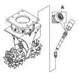
NOTICE! The drum cutter requires the additional *Tool Drain Kit* installed on the DXR because of the internal oil leakage in ER50.
