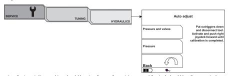
For auto adjustment, the machine should be standing on the outriggers and the tool should be disconnected.
