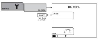
The gauge shows the oil level in percentage with even tens. Hold the selection key down to refill oil. The pump will shut off automatically when the tank is full.
