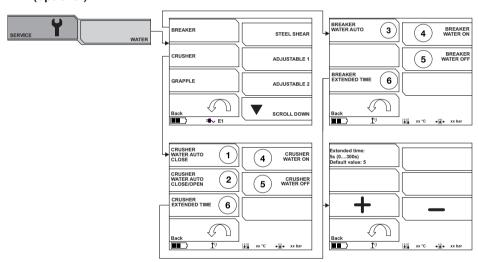
DXR equipped with a Dust Reduction kit enables the water function. The function can be activated together with various tools.
