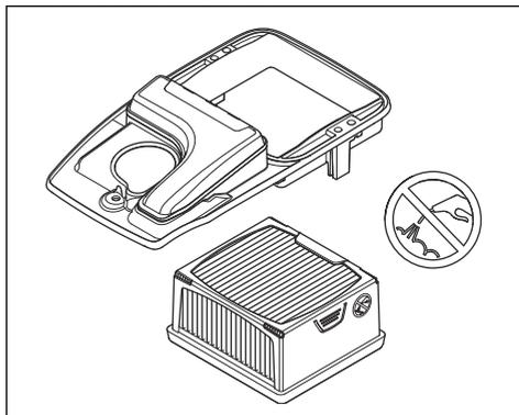
3. Loosen the 2 screws on the air filter pulley and remove it.
