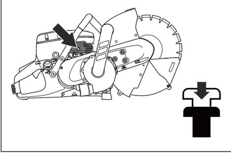
4. Push the air purge bulb 6 times until it is fully filled with fuel.
