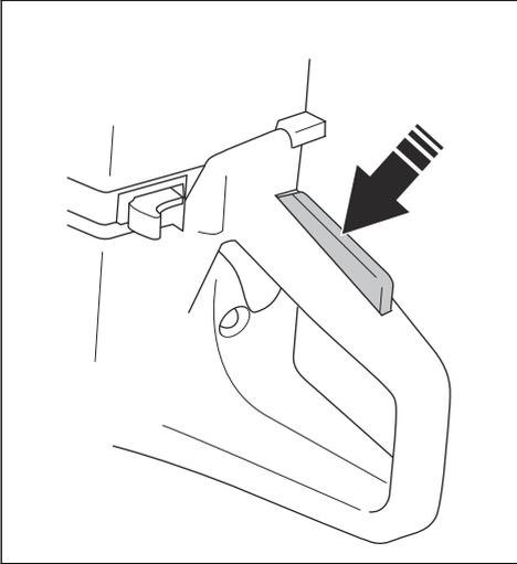
3. Make sure that the throttle trigger and throttle lockout move freely and that the return springs work correctly.
