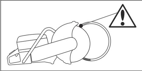
4. Move to side II and cut from section I to bottom of the pipe.
