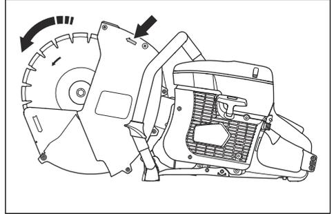
3. Make sure that the arrows on the blade guard and the cutting blade show the same direction.
