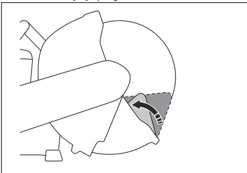
4. Make sure that the blade guard can be pushed in and return instantly by spring force.
