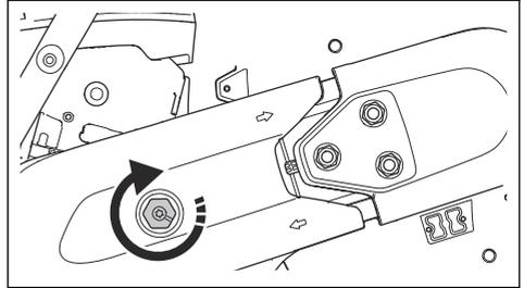
3. Jiggle the blade guard (A) up and down 3–5 times. Tighten the nuts (B).
