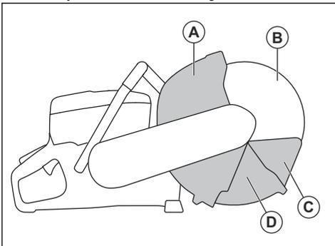
2. Make sure that the blade guard (A), the blade guard extender (D) and the dust shield (C) do not have cracks or other damage.
