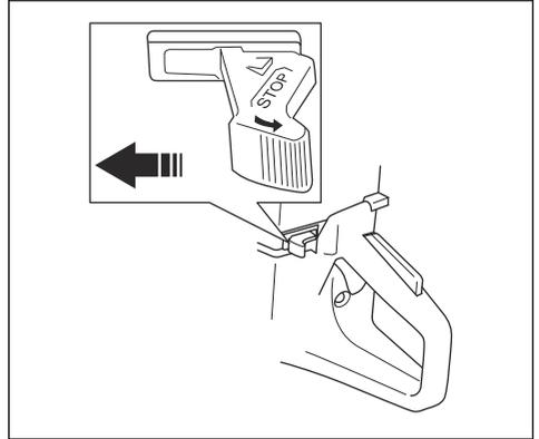
2. Pull the choke control fully and get the start throttle position.
