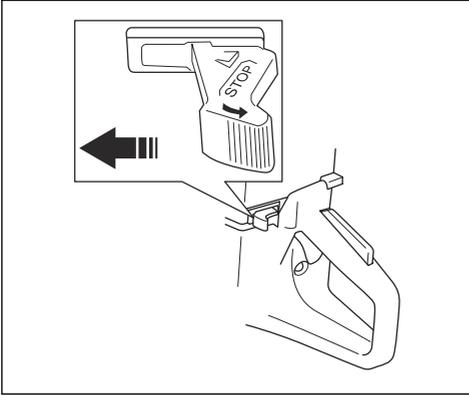
2. Pull the choke control fully and get the start throttle position.
