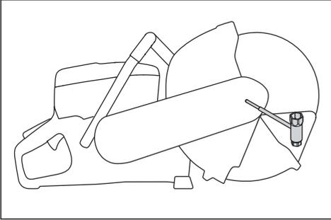
4. Tighten the bolt to 30 Nm (18.5 ft-lbs).
