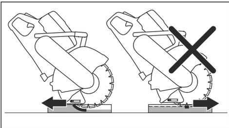
Push the cutting blade to the full cutting depth at the top/ front of the cut and move the cutting blade slowly down/rear. This decreases the temperature of the cutting blade and helps to collect the dust.
