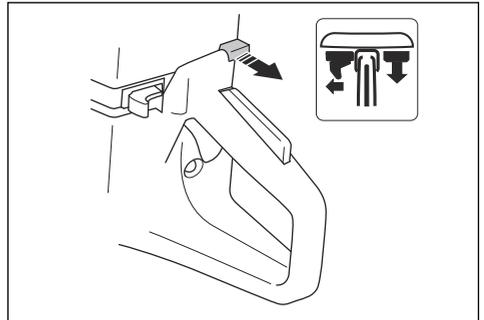
3. Push the decompression valve to decrease the pressure in the cylinder. The decompression valve goes back to its initial position when the product starts.
