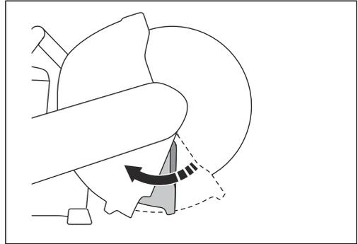
5. Replace the cutting blade and the blade guard if they are damaged. Replace the blade guard extender, the dust shield or their springs if they are detected and not returning instantly when pushed in.
