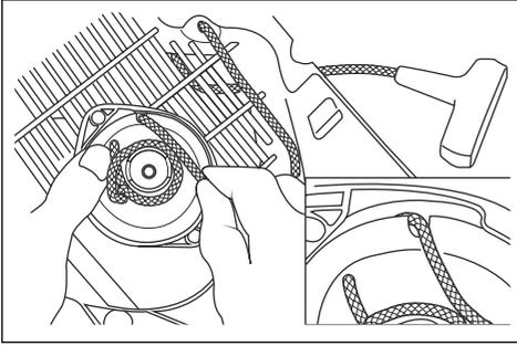
2. Let the rope pulley rotate slowly in the opposite direction to release the spring tension.
