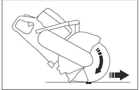
Never move the product when the cutting equipment is rotating. Gyroscopic forces can obstruct the intended movement
