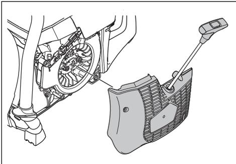
2. Keep the position of the starter rope and put the starter against the product.
