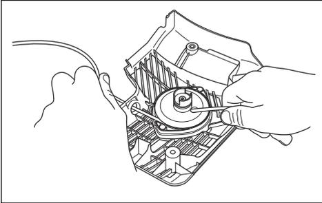
6. Attach the starter rope to the rope pulley.
