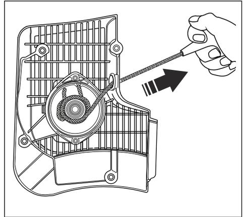
**Note:** The starter knob goes to its correct start position after adjusting the tension of the recoil spring.
