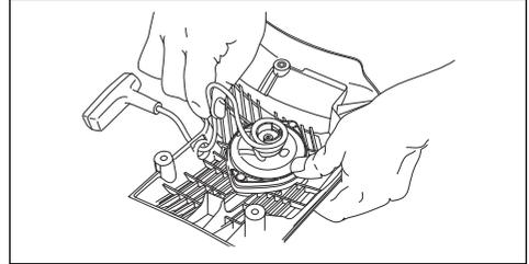
2. Pull the starter knob to adjust the tension of the recoil spring.
