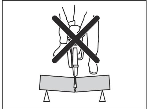
If the blade is pinched or stalled in the kickback zone, the reactive force will push the power cutter up and back towards the user in a rotating motion causing serious or even fatal injury. Be alert for potential movement of the work piece. If the work piece is not properly supported and shifts as you cut, it might pinch the blade and cause a kick back.
