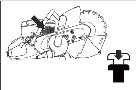
4. Push the choke control to disable the choke. The start throttle stays in position.
