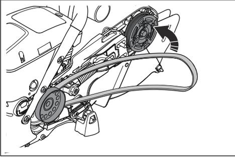
6. Make sure that the drive belt is put in correct position.
