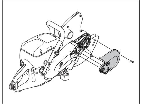
3. Remove the 2 screws on the rear belt guard. Remove the belt guard.
