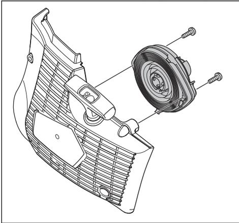
2. Push the 2 brackets on the snap locks with a screwdriver.
