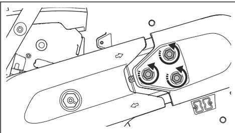
2. Turn the adjuster screw clockwise to increase the tension of the drive belt.
