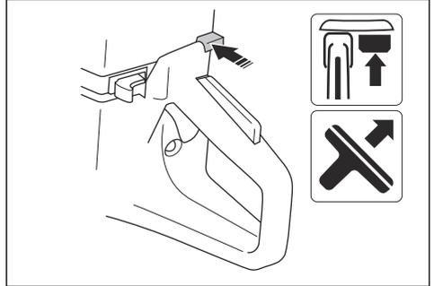
9. Push the throttle trigger to disengage the start throttle and set the product at idle speed.
