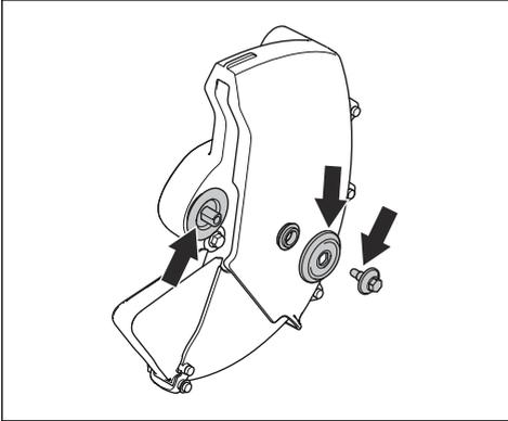
2. Make sure that the areas of contact on the cutting blade and the flange washers are not damaged.
