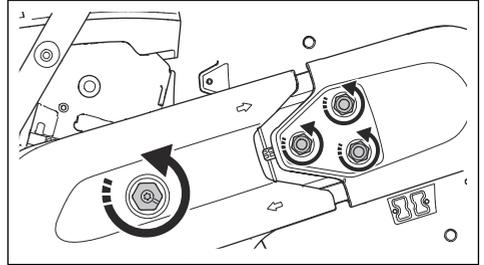
2. Remove the screw and the nuts. Remove the front belt guard.
