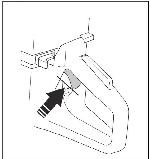
2. Push the throttle lockout and make sure it goes back when you release it.
