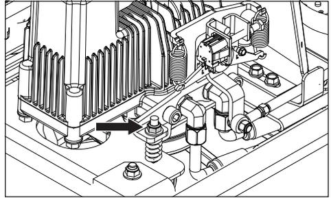
Tighten the nut to bias the unit toward reverse and loosen the nut to bias it forward. During adjustment of the nut, bump the controls into forward and/or reverse and let the controls snap back to neutral. When the wheel is stationary at the same time as the operator controls are in a neutral, tighten the socket cap screws to  $101 \pm 20$  Nm ( $75 \pm 15$  ft-lb). If the wheel continues to move, further adjustment is required.
