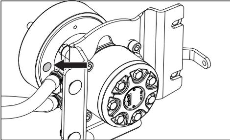
4. Using a brake spoon, turn the brake adjuster towards the front of the unit until the brake begins to engage. The adjuster should then be backed off three clicks.
