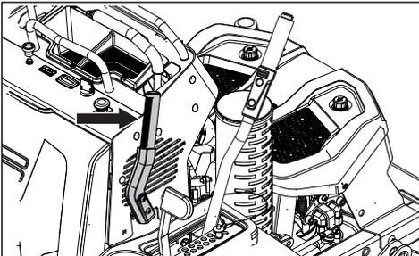
The park brake is found on the right side of the control console. Pull the lever back to engage the brake and push forward to release it.
