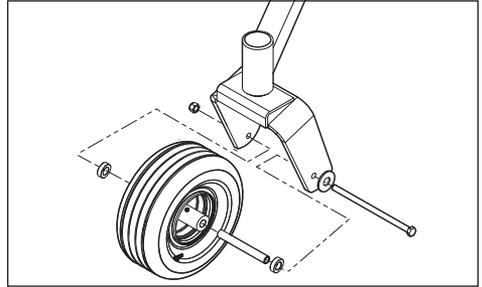
Check every 200 hours. Check that wheels rotate freely.
