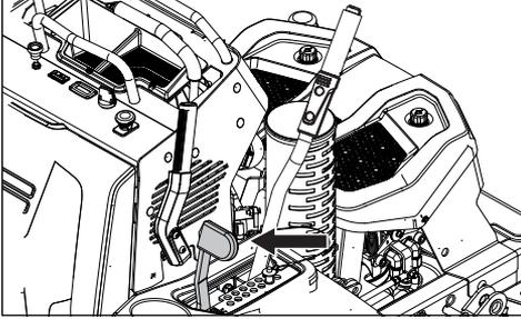
The transport latch will set the deck to the transport height of 5" when the lift lever is pulled back. The latch can also be used to mow at the 5" cutting height.
