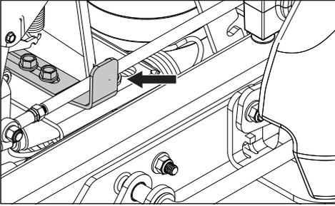
The hydraulic release allows the mower to be moved by hand when not running. See **Moving Machine By Hand** in the *Maintenance* section.
