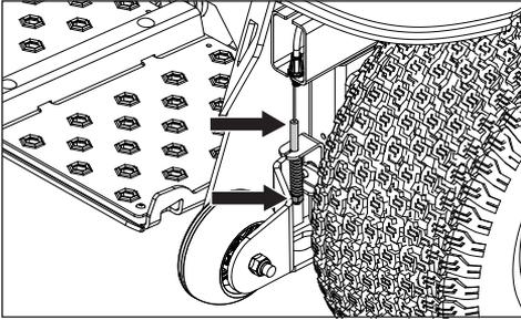
2. If the park brake pivot adjustment is not sufficient, the brake drum may need adjustment. With the rear of the unit supported on jack stands, remove the wheels. Disengage the brake and set the pumps to bypass mode. See **Moving Machine By Hand** in the *Operation* section.
