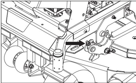
4. Turn the two outer blades to align with the deck front to rear. Reposition the rear mounting nuts up or down until the rear blade tips are positioned 6.4–9.5 mm (1/4"–3/8") higher in the rear than the center blade tips.
