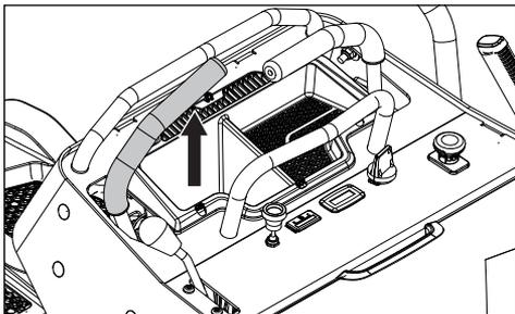
The left steering control is also the Operator Presence Control (OPC). The lever must be down and parallel with the right lever for operation.
