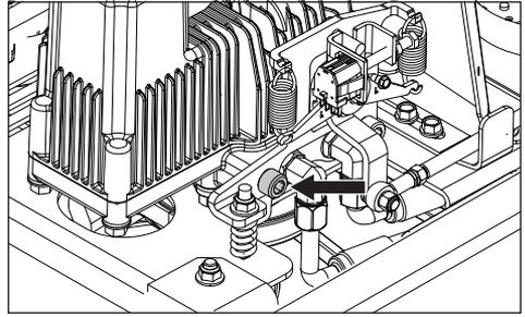
3. Start the unit. When unit is running, engage the OPC lever and release the park brake.
