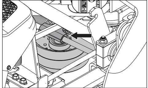
2. Remove the belt from around the clutch and the deck's front stacked pulley.
