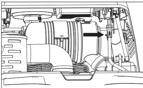
2. Adjust the nylon coupler until the desired speed is achieved. When the unit tracks straight and is at appropriate maximum forward speed, reinsert the retaining clip to lock the coupler in place.
