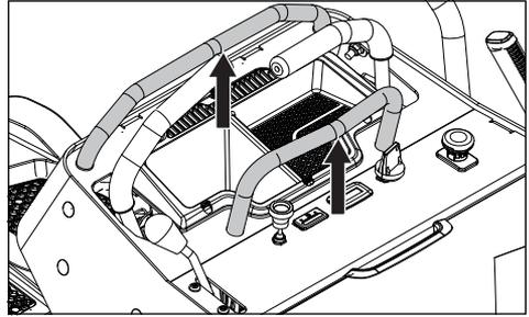
Located on the control panel, the stationary bars are fixed supports that assist the user when operating the steering controls.
