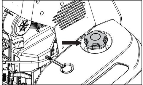
Read the safety instructions before refueling. The capacity for the tank is 24.6 litres (6.5 gallons).
