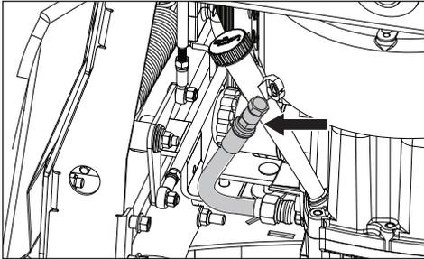
5. Route the drain hose down through the hole in the frame.
