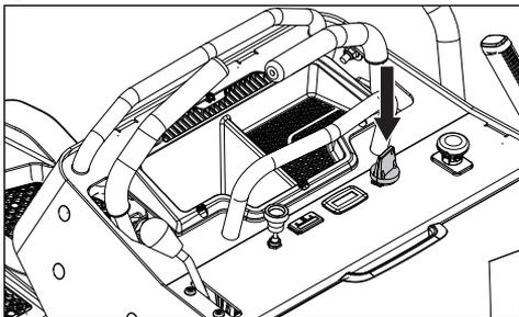
The ignition switch is used to start and stop the engine.
