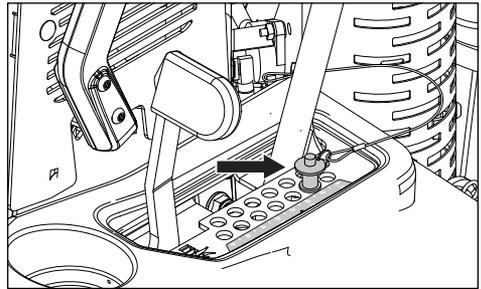
The cutting height can be set from 38 mm to 127 mm (1-1/2" to 5").
