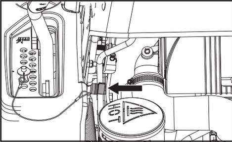
The valve is off when the handle tab is turned perpendicular to the fuel line.
