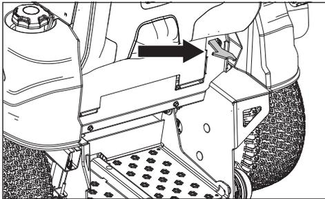
To remove, tip the lowered cushion up slightly and lift the back edge up.
