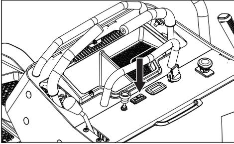
The fuel gauge for the fuel tank is located on the control panel. Sensors will indicate fuel levels. The meter will flash yellow when the tank level is approximately 3.8 litres (1.0 gallons).
