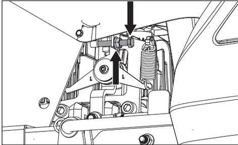
3. Adjust the neutral bolt on the left side of the unit so the plunger on the neutral switch is flush with the surface of the switch.
