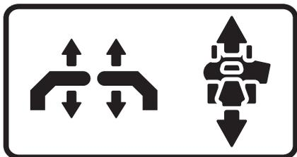
Pull back slightly on control levers, allowing the mower to move backwards. Release the control levers to the neutral position to stop the mower from moving.
