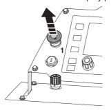
Reset the safe mode by turning Engine start switch to the STOP position and back to ignition on position.
