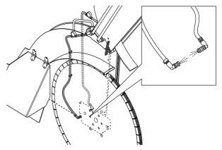
Test for adequate water supply. Low water flow will cause damage to diamond blades. Engage the Water safety switch on the control panel and open the Water valve.
