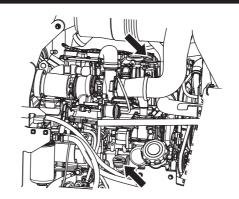
Refill the system at either of 2 locations on the engine.
