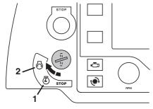
Press the machine stop and check that the engine stops.
