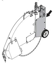
NOTICE! Do not operate this saw without the latch engaged and the bolt installed. Do not use if damaged. Do not operate this saw without the front-slider protection installed.
