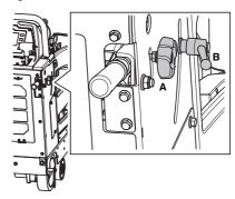
Lower the front guide and align the front guide, rear guide and the diamond blade with the line on the surface. The front guide is telescopic, adjust the length with the screws on the inside of the front guide.
