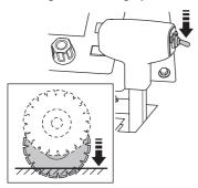
CAUTION! When lowering the blade into a partial cut, align the blade exactly with the cut to prevent damage to the blade.
