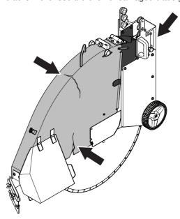
Clean the inside of the blade guard. Inspect the wear plates.
