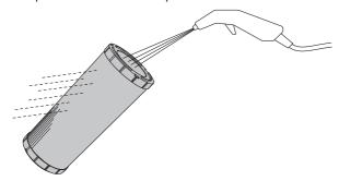
NOTICE! Do not exceed recommended air pressure. A higher air pressure will damage the air filter.
