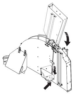
Always attach the front slider protection on the blade guard. Make sure it moves up/down freely.
