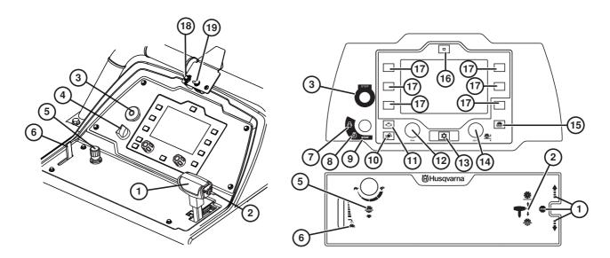
The control panel is the operator's link to the machine. From here the operator can control anything from engine rpm, cutting depth of the blade and read the current status of the engine and the machine.
