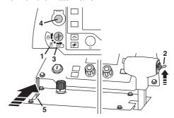
Loosen the blade guard front bolt and lift the blade guard latch
