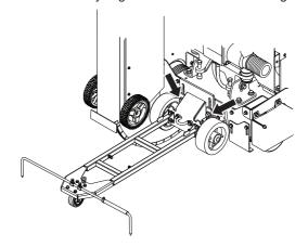
Set the desired cutting depth by rotating the Depth knob.
