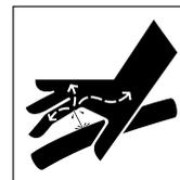
**Pressurized fluid can inject into the body**
