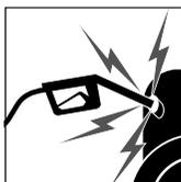
Static discharge during fueling can cause explosion
