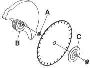
Lock the shaft. Insert a tool in the hole in the cutting head and rotate the blade until it is locked.
