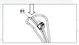
Before Switching on the BG-180EC, the front part of the grinding machine must be lifted by pushing the handgrip (1) down to floor level till the machine is approximately 10cm from the ground.
