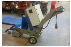
The traction wheels must be disconnected from the drive motors: pull out the locking pin of each rear wheel. The machine can now be pushed around on its wheels.
