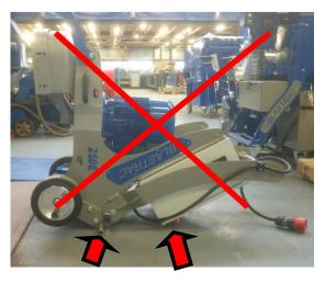
Lay the machine backwards on the handle and flip the bracket with the castor front wheel down.
