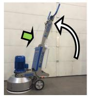
Before you tilt the machine back, make sure the electrical cable and dust hose cannot get damaged when you tilt the machine back.
