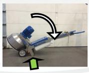
Tilt the machine back and lay down the machine so it is laying on the metal support underneath the electrical box. Make sure the machine will not fall back down. A second person can hold the handle down, to make sure the machine will not fall back down.
