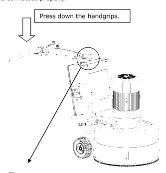
Use two pins when you tilt the machine back
