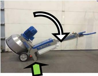
Tilt the machine back and lay down the machine so it is laying on the metal support underneath the electrical box. Make sure the machine will not fall back down. A second person can hold the handle down, to make sure the machine will not fall back down.
