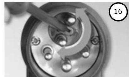
Using a Screwdriver the phases can be inverted
