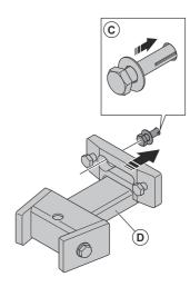
7. Attach the mounting bracket (D) to the anchor screw.
