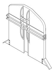
Blade guard that can be adjusted for near floor operatons.
