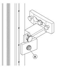
Adjust the distance between the cut line and the mounting brackets. The distance between the edge and the inner face of the cut must be (B) = 89 mm/3.5 in.
