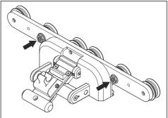
2. Attach the blade guard guide to the blade guard.
