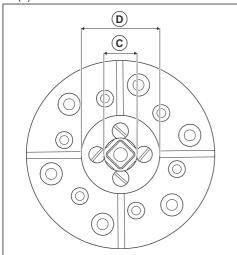
9. Assemble the flush cutting blade on the blade flange hub.
