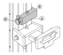
Make sure that the track holder is fully seated on the mounting brackets before you tighten the screw(A).
