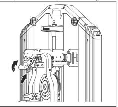
7. Connect the water hose from the outlet on the saw motor to the inlet on the blade flange hub.
