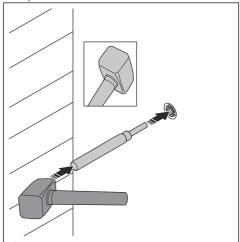
Put the M6S 12×70 (1/2 in.×2 in.) or equivalent anchor screw (C) into the hole.
