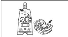
Push the ON/OFF button to start the remote control. This also starts the connected power tool, information is shown on the display.
