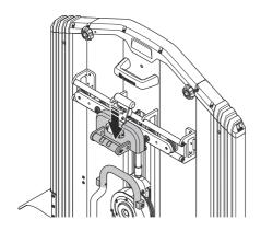
Make sure that plastic plugs are attached on the drain holes of the blade guard. Clean the drain holes after each operation.
