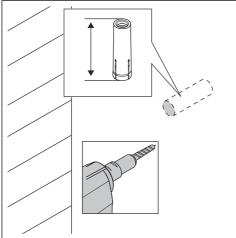
5. Use the mandrel and a hammer to install the expander.
