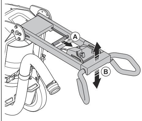
2. Adjust the handle (B) to an applicable operation height.
