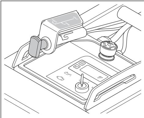
3. Push the product forward across the floor surface. Use the throttle control to adjust the speed between "MIN" and "MAX" while you operate the product.
