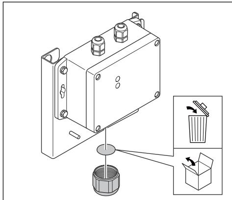
3. Install the new filter for the carbon monoxide detector in opposite sequence.
