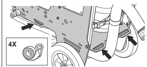
3. Attach and tighten the tie-down straps to the vehicle.
