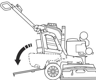
6. Make sure that the water tank cap is fully closed before you tilt the product.
