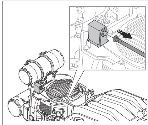
3. Remove the speed control servo and the clean out covers for the cylinder.
