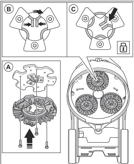
14. Push the center tabs together and rotate clockwise (B) to lock the tool plate to the grinding disc (C).
