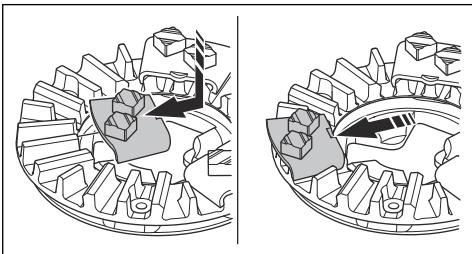
13. Attach the tool plate straight (A) on the grinding disc.
