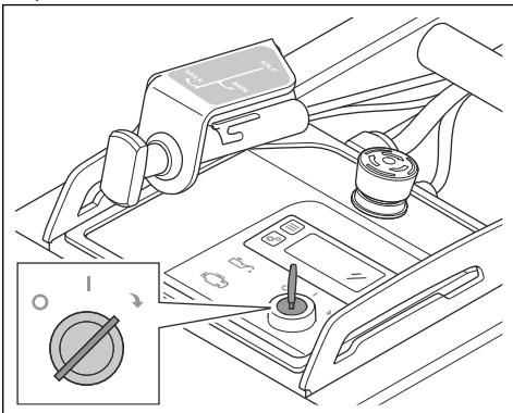
5. When the engine starts, immediately release the ignition key. The ignition key goes to the "1" position.
