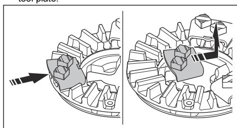
12. Attach new diamond tools to the tool plate with a soft hit of the hammer.
