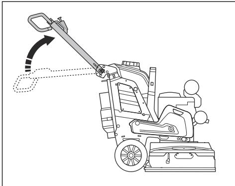
1. Pull the lock lever (A) on the handle in the direction of the control panel and hold it in this position.
