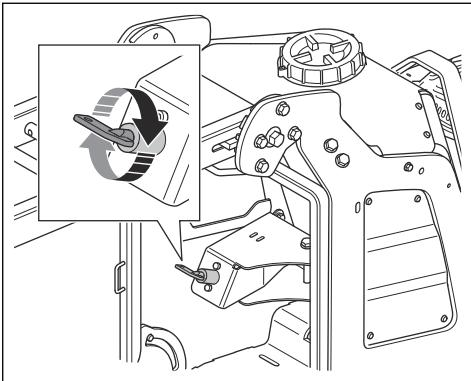
3. Pull out and turn the throttle control to idle speed for the engine. Refer to *Rpm for the engine on page 5*.
