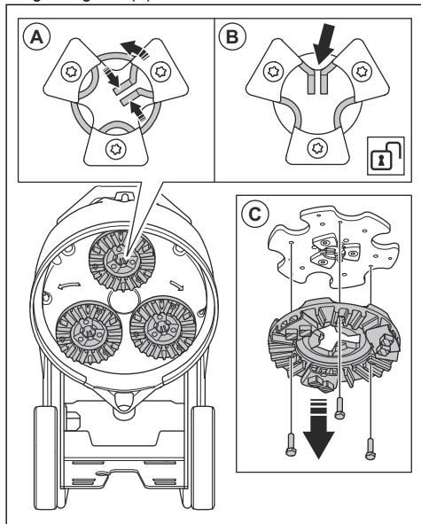
10. Pull the tool plate straight out (C) to remove the tool plate from the grinding disc.
