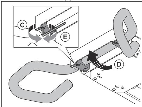
5. Adjust the handlebar (D) to an applicable operation height.
