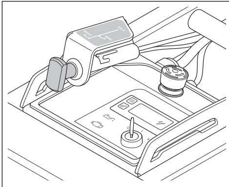
2. Turn the propane tank valve clockwise until it stops to stop the propane supply to the engine.
