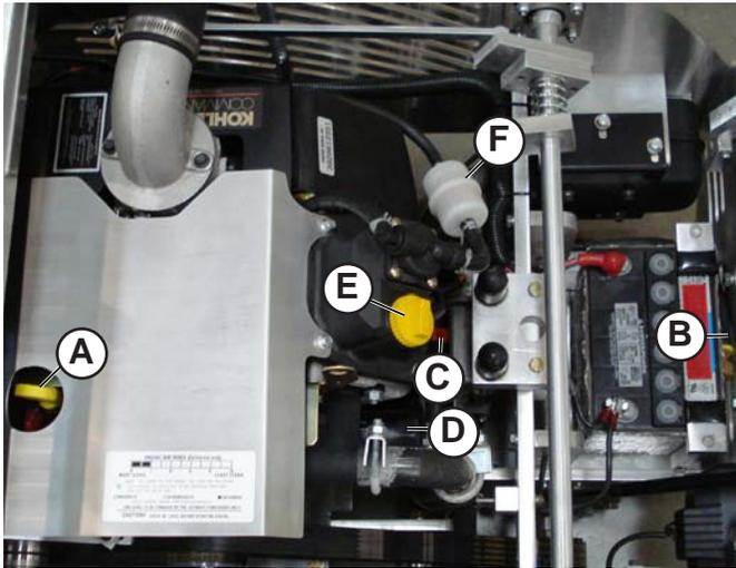
The oil drain hose (B) is located at the front of the saw by the battery.
