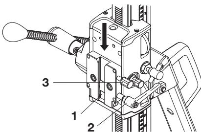
Use top positioned locking screw (3) only together with DMS 240.
